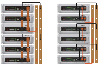
Figure 5-1 Schematic diagram of power cable connection
