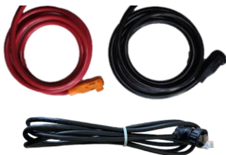
Model: RW-M6.1-PCable Details: Pair of 4AWG DC power cable and RJ45 communication cable connect with hybrid inverter, one end has a waterproof terminal . The cable length can be customized based on customer requirements, default length is 1500mm.
